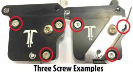
· Housing has three screws securing the lid
